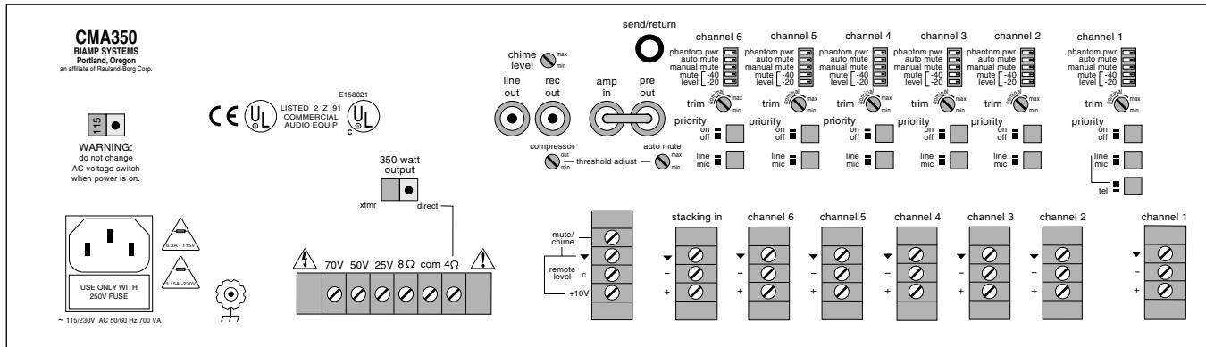
**Power Entrance:** This receptacle accepts a 3-prong AC power cord. **WARNING: DO NOT REMOVE OR DEFEAT THE GROUND PRONG, AS THIS CONSTITUTES A SHOCK HAZARD.** The removable lower portion of the receptacle holds the AC fuse. **NOTE:** See AC Fuse on page 7 for replacement by qualified personnel. A chassis ground post is provided (next to the receptacle) for system grounding.
