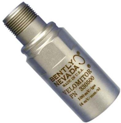
Bently Nevada™ Velomitor Piezo-velocity Sensors are designed to measure absolute (relative to free space) bearing housing, casing, or structural vibration. The 330500 is a specialized piezoelectric accelerometer that incorporates embedded integrated electronics in a solid-state design.
