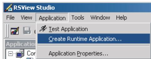
7. Compile the project, download it to the terminal, and run the project. If successful, the communication status LED's illuminate on the 2711P-RN15S module.
