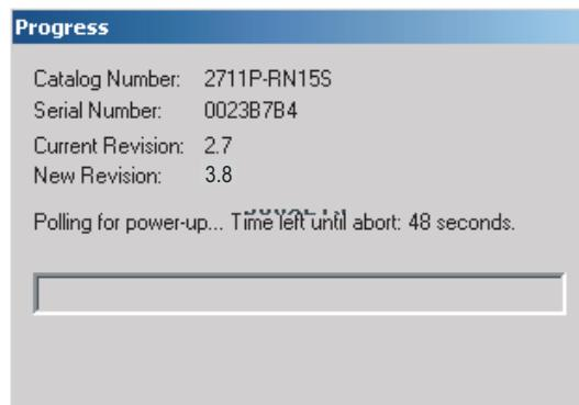
When the terminal recycles power, the Control Flash firmware upgrade utility verifies the communication card update.
