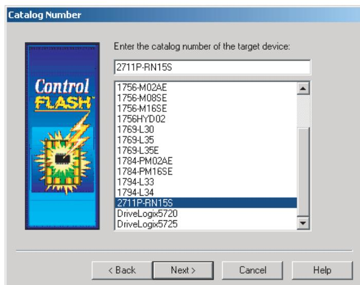
3. Select 2711P-RN15S to upgrade via an Ethernet or ControlNet network and click OK.
