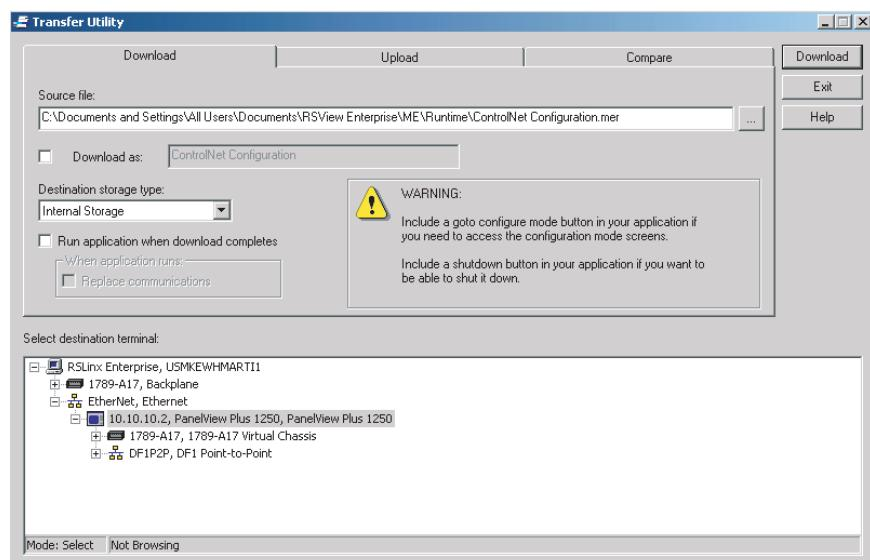
A sample .MER has been created to configure the 2711P-RN15S as Node 2 on a ControlNet network. This application is located on Technote A103053983 on the Rockwell Automation Technical Support Knowledgebase at <http://support.rockwellautomation.com>. Download and run ControlNet Configuration.mer on the PanelView Plus or PanelView Plus CE.
