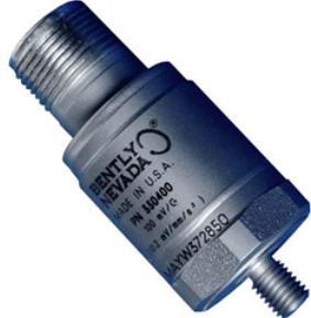
These accelerometers are intended for critical machinery applications where casing acceleration measurements are required, such as gear mesh monitoring. The 330400 is designed to address the requirements of American Petroleum Institute Standard 670 for accelerometers. It provides an amplitude range of 50 g peak and a sensitivity of 100 mV/g. The 330425 is identical except it provides a larger amplitude range (75 g peak) and a sensitivity of 25 mV/g.
