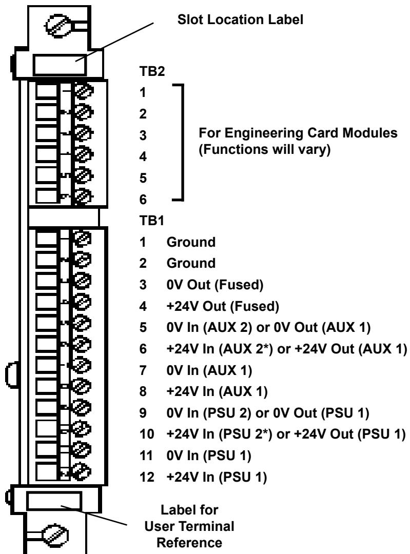
\* PSU 1 and PSU 2 (and AUX 1 and AUX 2) must be compatible with parallel connection.
