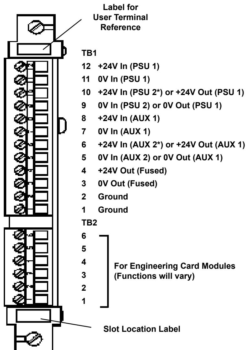
\* PSU 1 and PSU 2 (and AUX 1 and AUX 2) must be compatible with parallel connection.
