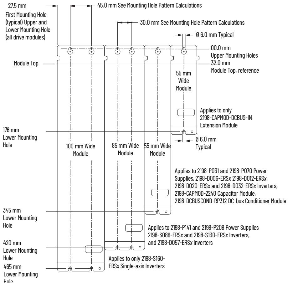
When your Kinetix 5700 system configuration includes 2198-S263-ERSx or 2198-S312-ERSx single-axis inverters, see the Kinetix 5700 Servo Drives User Manual, publication [2198-UM002](#), for those mounting hole patterns.
