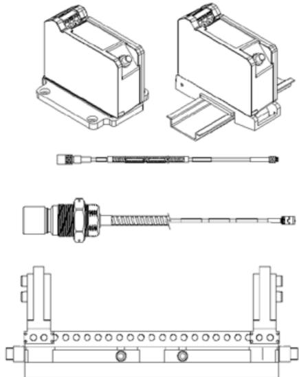
The 3300 XL 25 mm Transducer System consists of a separate 25 mm probe, an extension cable, and a 3300 XL 25 mm Proximity Sensor. The 0.787 V/mm (20 mV/mil) output gives this system a linear range of 12.7 mm (500 mils). Based on this linear range, the 3300 XL 25 mm Transducer System is suitable for measuring differential expansion (DE) on mid-size to large steam turbine generators caused by the difference in growth rates between the turbine rotor and the machine stator (casing).
