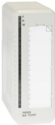
The AI835/AI835A provides 8 differential input channels for Thermocouple/mV measurements. Measurement ranges configurable per channel are: -30 mV to +75 mV linear, or TC Types B, C, E, J, K, N, R, S and T, for AI835A also D, L and U.
