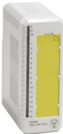
The DO880 is a 16 channel 24 V digital output module for single or redundant application. The maximum continuous output current per channel is 0.5 A. The outputs are current limited and protected against over temperature. Each output channel consists of a current limited and over temperature protected high side driver, EMC protection components, inductive load suppression, output state indication LED and an isolation barrier to the Modulebus.
