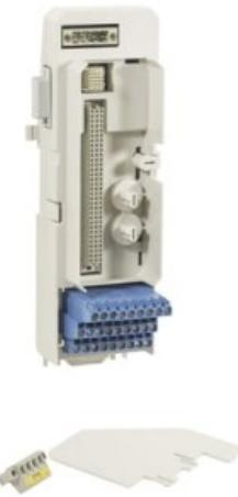
The TU890 is a compact MTU for the S800 I/O. The MTU is a passive unit used for connecting the field wiring and power supply to the I/O modules. It also contains a part of the ModuleBus. The TU890 MTU has gray terminals for field signals and process voltage connections. The maximum rated voltage is 50 V, and the maximum rated current is 2 A per channel, but these are primarily constrained to specific values by the design of the I/O modules for their certified application.
