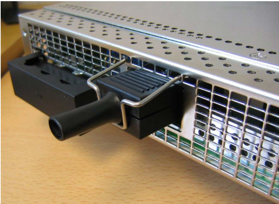
Figure 3 AC Power Connectors and Retaining Clips
