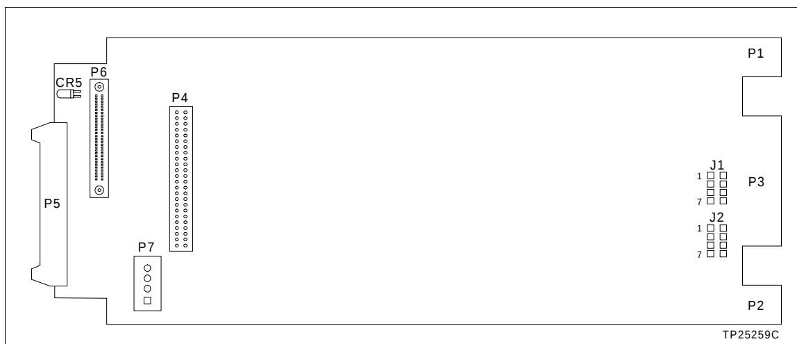
Figure 3-2. IMMPIO1 Jumper Locations
